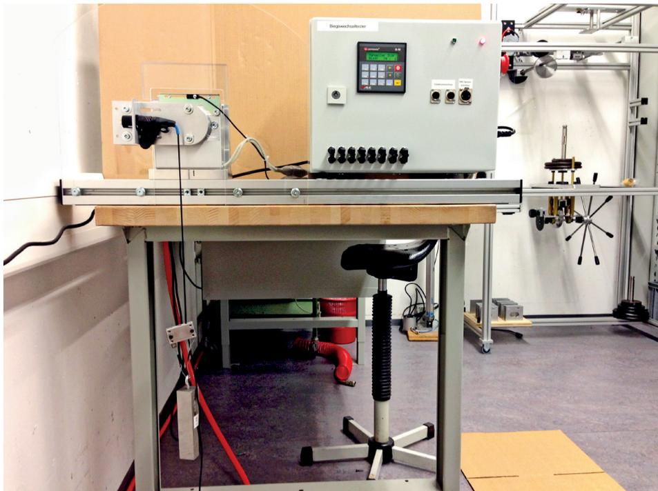
figure 8.b: Test Equipment and Fixture for flexing test
