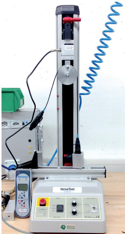
figure 3: Equipment for examination of cable retention
