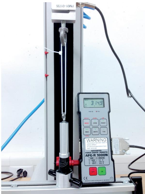
figure 4: Equipment for examination of locking mechanism
