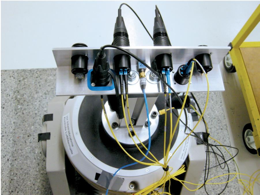
figure 2.b: : Vibration equipment and test cable arrangement
