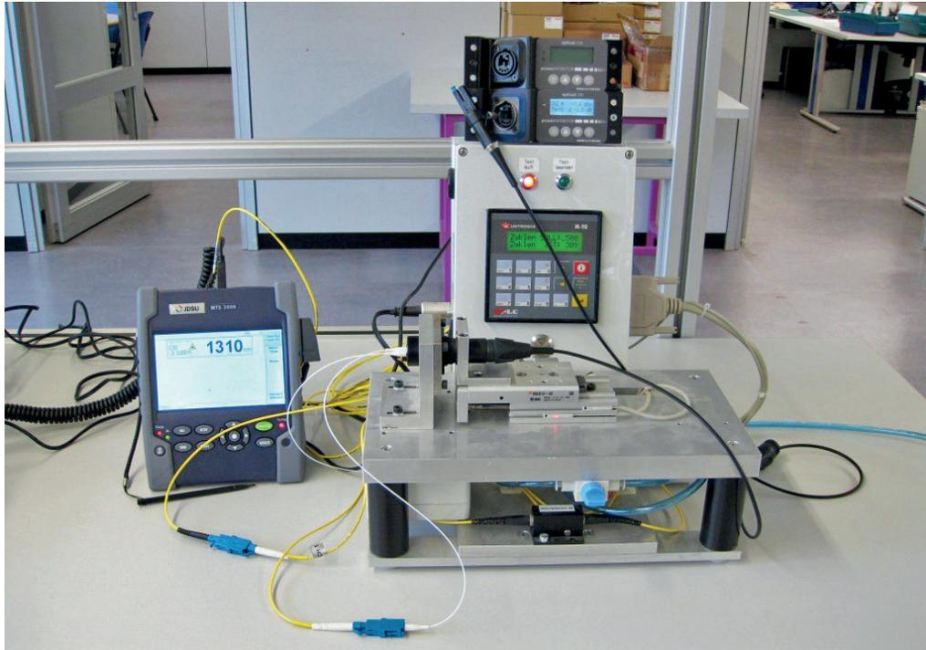
figure 6.a: measuring setup for durability and lifetime test
