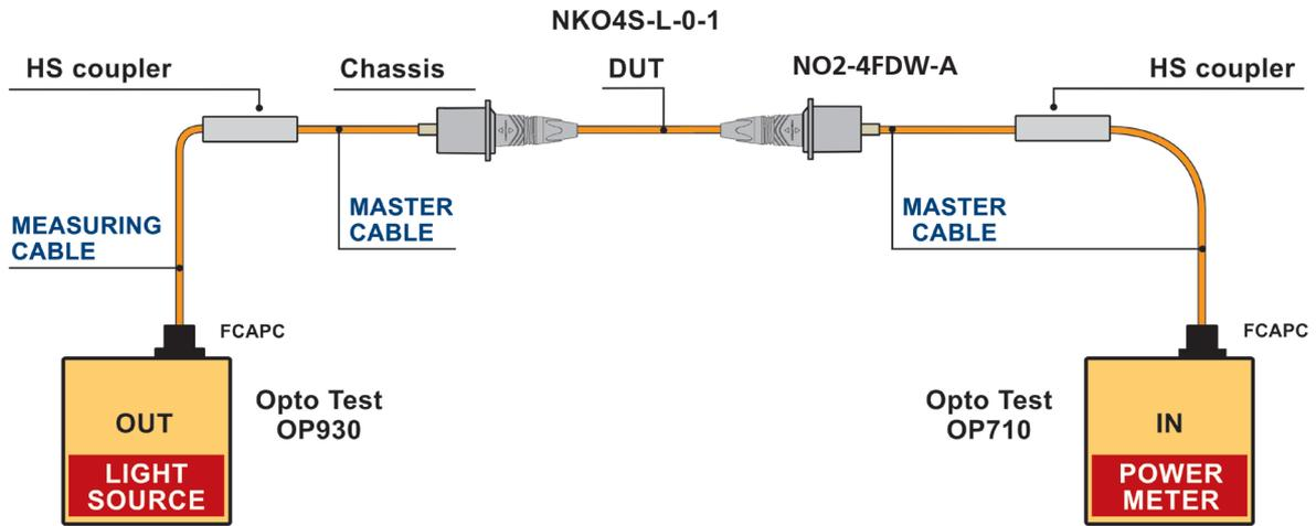
figure 1.b.: Simplified measuring arrangement
