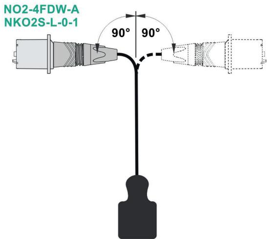
figure 8.a: Principle of Test according to IEC 61300-2-44 (IEC 61300-3-4)
