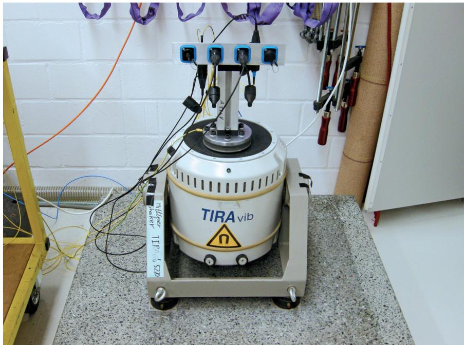
figure 2.a: Vibration equipment and test cable arrangement
