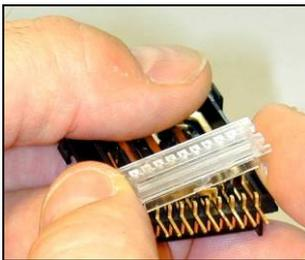
Then remove the cover with a tiny grip at the side and carefully
