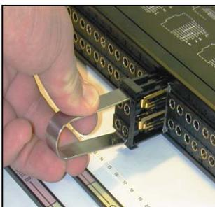
Pull one module out of the casing using the supplied disassembling pliers
