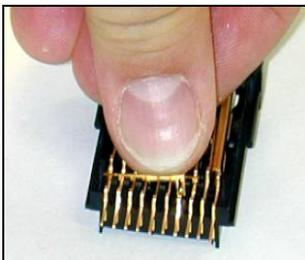
Insert new bars carefully by pressing them in parallel at both ends.
