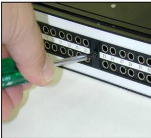
Remove Front Panel by unscrewing the 3 black cross-recessed screws (M3x8 Taptite), remove the two side-stops.
