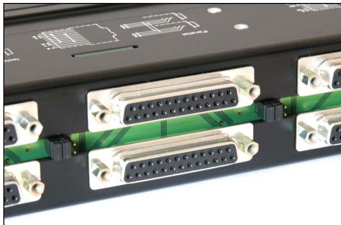
25 pin Sub-D connector terminal (SD25)
