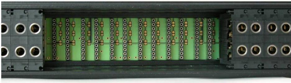
Each Sub-D group is configured by its own jumper block. The flexible grounding system provides the following alternatives to choose from:
