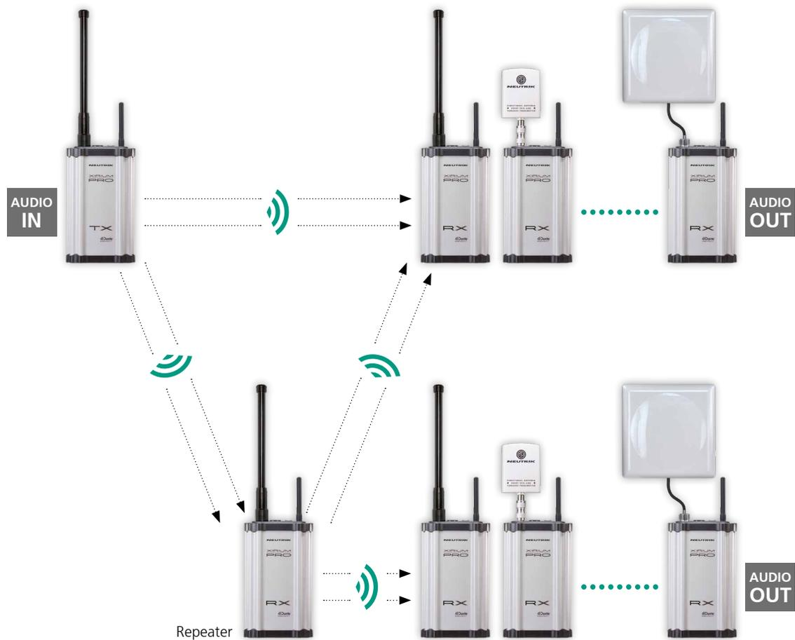
... using the repeater as a redundant audio source (extended true diversity).
